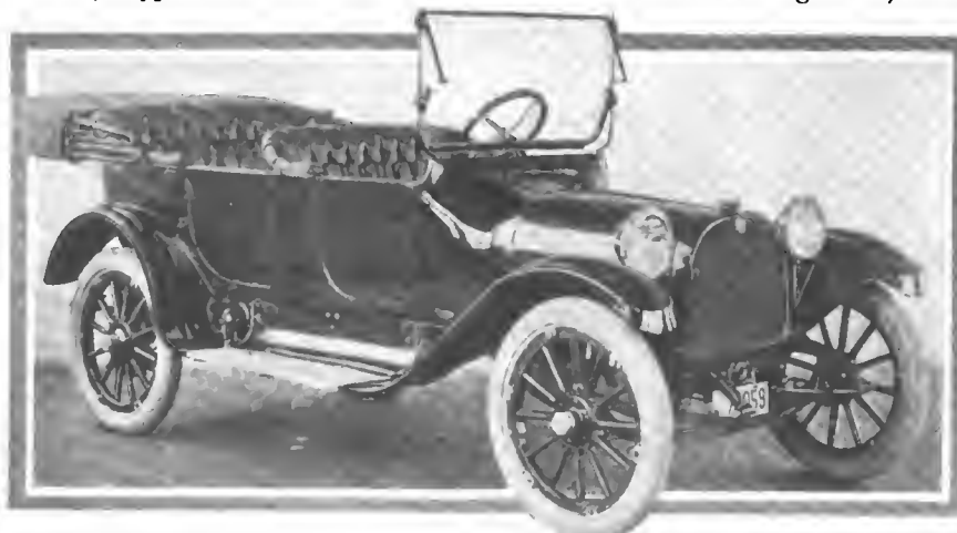
New Dodge car, showing streamline five-passenger body, rounded-over edges on radiator, smooth doors, etc.
